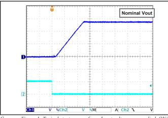
Common Figure 1: Typical startup waveform. Input voltage pre-applied, ON/ OFF Pin on Ch 2.
