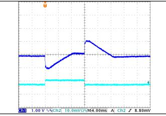
Figure 5: Output voltage response to step-change in load current (50%-75%-50% of Iout(max);  $dI/dt = 0.1A/\mu s$ . Load cap: 100 $\mu F$  electrolytic cap and  $1\mu F$ ceramic cap. Ch 1: Vout, Ch 2: Iout (10 A/div).
