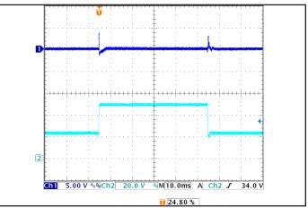
Figure 6: Output voltage response to step-change in input voltage (250 V/ms), at Max. load current. Load cap:  $100\mu$ F electrolytic cap and  $1\mu$ F ceramic cap.Ch 1: Vout, Ch 2: Vin.
