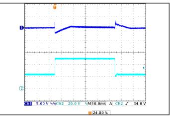
Figure 6: Output voltage response to step-change in input voltage (250 V/ms), at Max. load current.Load cap: 100µF electrolytic cap and 1µF ceramic cap.Ch 1: Vout, Ch 2: Vin.
