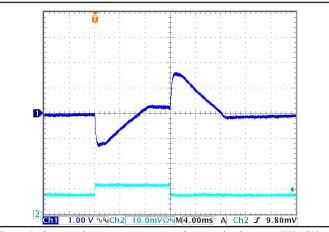
Figure 5: Output voltage response to step-change in load current (50%-75%-50% of Iout(max);  $dI/dt = 0.1A/\mu s$ . Load cap:  $100\mu F$  electrolytic cap and  $1\mu F$  ceramic cap. Ch 1: Vout, Ch 2: Iout (5 A/div).
